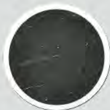
No Retrofit System Uncontrolled Diesel Exhaust
