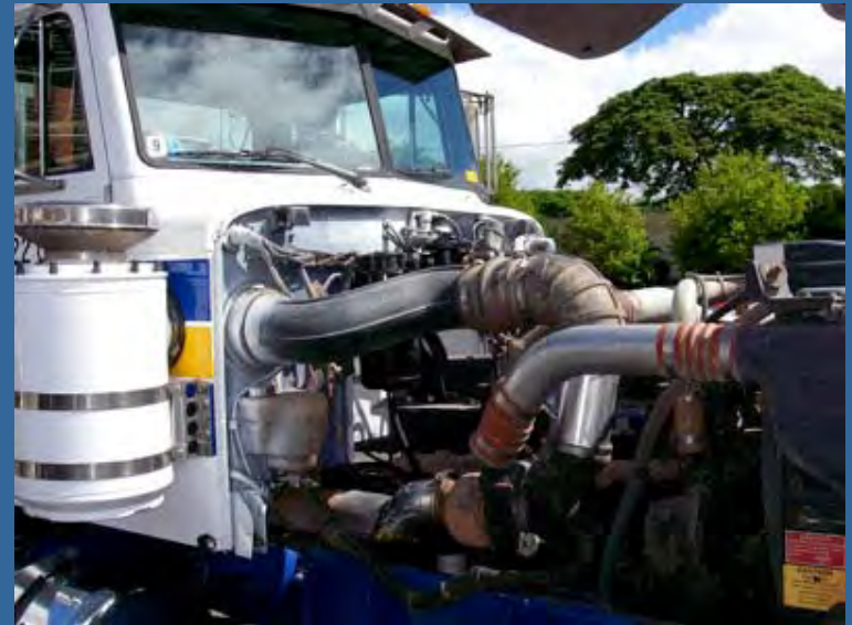
Closed crankcase ventilation system on a Grace Pacific truck.
